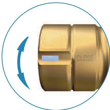
To lock the One-Step Insertion Sleeve, the inner and outer sleeve are twisted in opposite directions until the mark on the inner sleeve lines up with the “close” mark on the outer sleeve.
