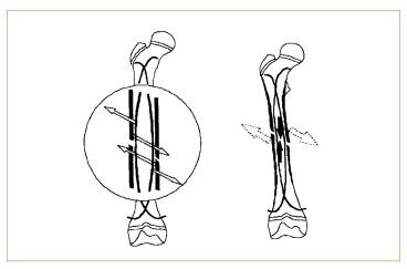
Implants carry load parallel to the axis of the bone and shear displacement between fracture elements is prevented.
