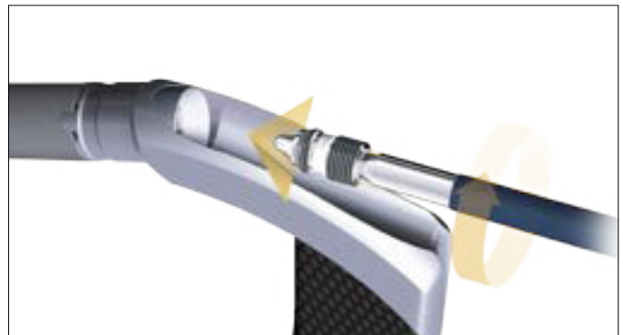
Fig. 56 Set Screw insertion
