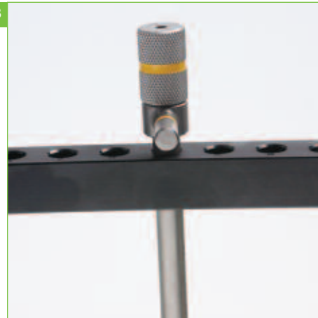
Thread 3.8 mm drill guide through sheath.
