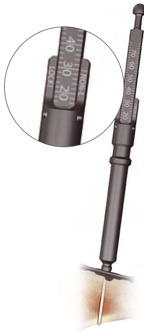
Step 3 Take a direct reading from the NON-L line.
